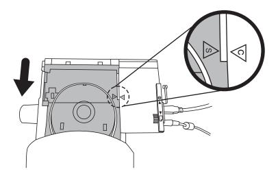
8. Reattach the Autoloader to the printer and slide the Printer Mode Switch back to the "disc" position
